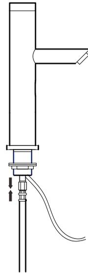
Screw the flexihose on to the bottom of the threaded tube, hand tighten only.
