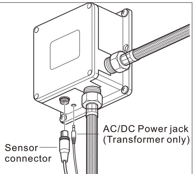
Hold the plug not the wire to connect and dis-connect.
