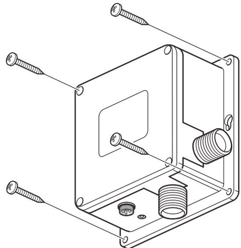
Screw control box in a suitable position under the basin making sure flexihose and control cable can reach.
