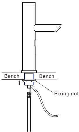
Tighten the fixing nut to secure tap to bench top (do not over tighten as this may damage bench top) Do not tighten the threaded tube.
