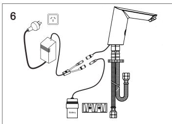
AC/DC Transformer with battery back up: Fix bracket to wall and connect battery box to transformer plug then connect other transformer plug to tap control cable. Plug into socket.
