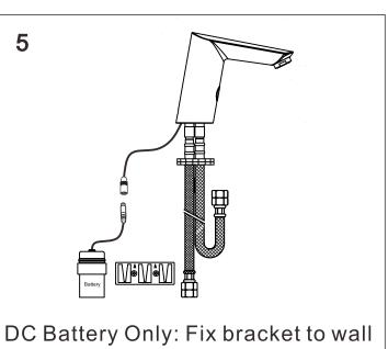
DC Battery Only: Fix bracket to wall and connect battery box to control cable.
